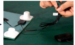
4, Input cable connect with led driver and the light on.
