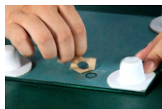
2, Fix the sensor with 3M tape on the back of the mirror.
